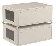
A pair of Blizzard 52.150 Landscape enclosures with 52.SK Stacking Kit. The kit maintains the required 75mm airflow gap between the two enclosures
