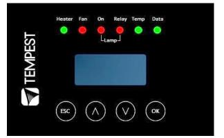
DEC 3.3's patented Goldilocks<sup>™</sup> algorithm uses a combination of sensors, heaters and fans to maintain a safe operating temperature and a safe relative humidity level that will not allow condensation to take place.
