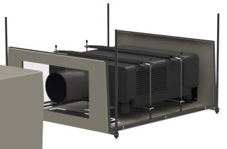
When installed hanging, the cover is removed by lifting slightly and sliding to front (shown) or back. Allow at least 50mm (2in) between enclosure top and any overhang.
