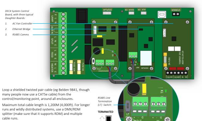
Use the termination switch to terminate each RS485 cable run at the last enclosure on each run.
