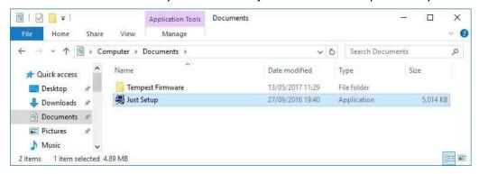
3. Run JUST and select the top left USB connection Icon. Select the DEC4 from the Connection Details option and click the connect/plug Icon. Having connected, close the connection window.
