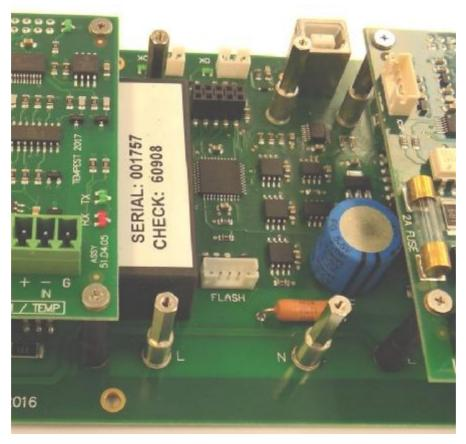
3. Place heat-shrink insulation sleeves over the front two posts and stand-offs
