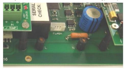
2. Screw in 4 stand-off pillars, supplied in mounting kit.
