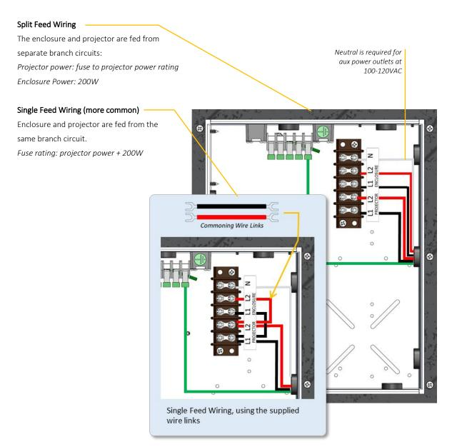
For clarity, blower power supply (Zen 3xx – 5xx) and internal wiring are not shown
