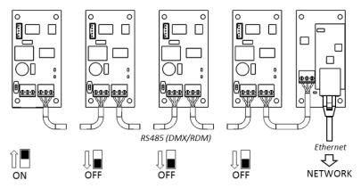
3. TSM/TEMP Control of a single enclosure via Ethernet
