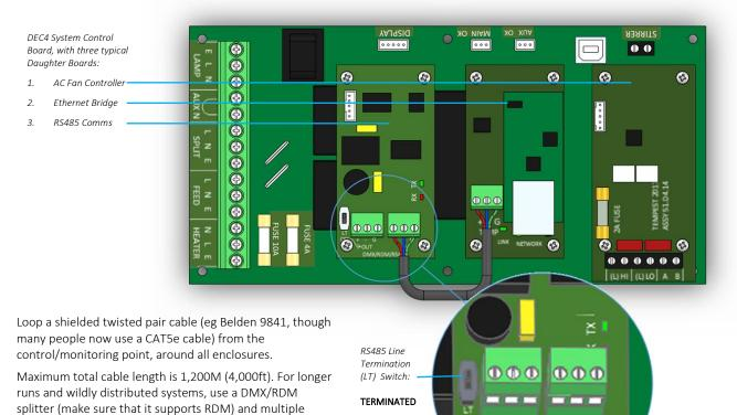
Use the termination switch to terminate each RS485 cable run at the last enclosure on each run.
