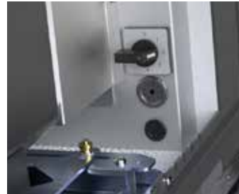
Simply preselect one of standard Zen's four fan speeds - the thermostat in the projector exhaust airflow starts the blower as soon as the projector comes out of standby.
