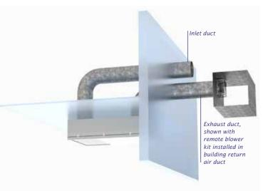
If it is impractical to bring inlet air from a remote location, use a length of padded flexible hose (250mm/10in ID) in an 'S' configuration to draw in air and muffle any noise escaping through the air inlet path.
