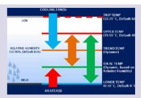
sure just right by using heaters to raise the air temperature when needed, adapting constantly to prevent deadly condensation.
