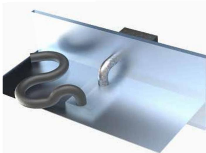
If it is impractical to bring inlet air from a remote location, use a length of padded flexible hose (250mm/10in ID) in an 'S' configuration to draw in air and muffle any noise escaping through the air inlet path.
