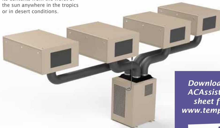
Rendering: A group of four Blizzard 52.150 enclosures, with AC Assist Cooler and flexible hose manifold. The cooler may be located anywhere within 5m (16ft) of the enclosure air inlet. Allow at least 500mm (20in) below the enclosure(s) for the cooler hose and its bend radius.
