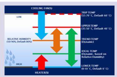
Goldilocks uses a heater to maintain a minimum temperature in cold climates.
