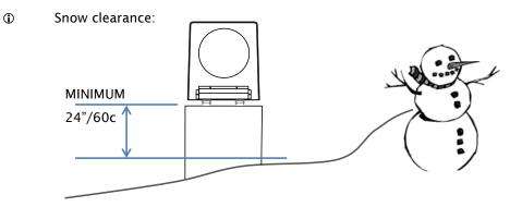
① Allow at least 24"/60cm clearance behind enclosure for access and ventilation.
