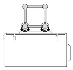
Use two clamps to mount to a pipe, or to mount from a truss at an angle. Use four clamps to mount parallel to a truss.
