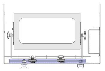
Adjust the position of the spring bolts in the Unistrut to correspond with two of the mounting holes in the Atomic Strobe yoke.
