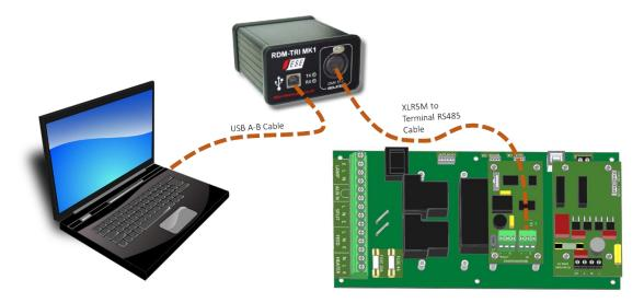
4. Power up the target SCB, ideally with mains power, or alternatively, with a USB power adaptor connected to the USB Port on the SCB.
