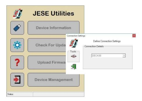
**4.** From the main window, select the 'Upload Firmware' option. Select the file Icon and navigate to the firmware file to upload
