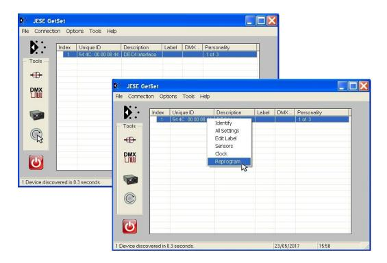
In the Firmware upload handler, search for a file to upload by clicking the file icon. Find and select the file to load and click the Open button.
