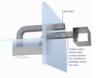
If it is impractical to bring inlet air from a remote location, use a length of padded flexible hose (250mm/10in ID) in an 'S' configuration to draw in air and muffle any noise escaping through the air inlet path.
