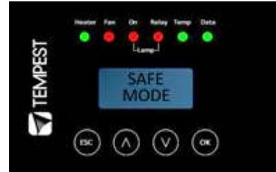
In SAFE MODE, the normal Goldilocks operation is temporarily suspended, and the enclosure works to return the internal environment to a condition from which normal operation may be resumed.
