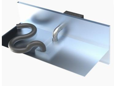
If it is impractical to bring inlet air from a remote location, use a length of padded flexible hose (250mm/10in ID) in an 'S' configuration to draw in air and muffle any noise escaping through the air inlet path.
