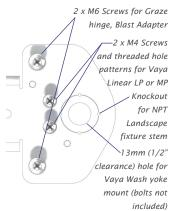
Compact Burst fixture — note that the wall offset increases by 2.5in [6cm] with the adapter plate fitted.
