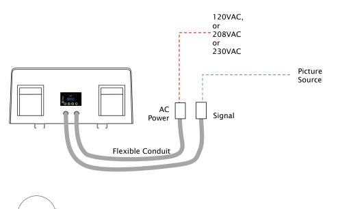
The conduit entry holes accept US  $\frac{1}{2}$ " conduit fittings, and international 20-22mm (OD) conduit fittings.
