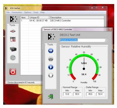
This view shows a single DEC3.2 test unit that has been correctly discovered and labeled by the GetSet software suite, and a log of RDM messages.
