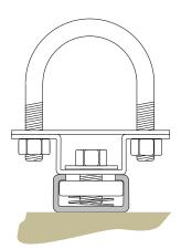
**4900.MC** Stainless Steel Unistrut channel nut, bolt and pipe clamp, for pipes 1.5" (38mm) to 2" (50mm) OD. Four required per enclosure.
