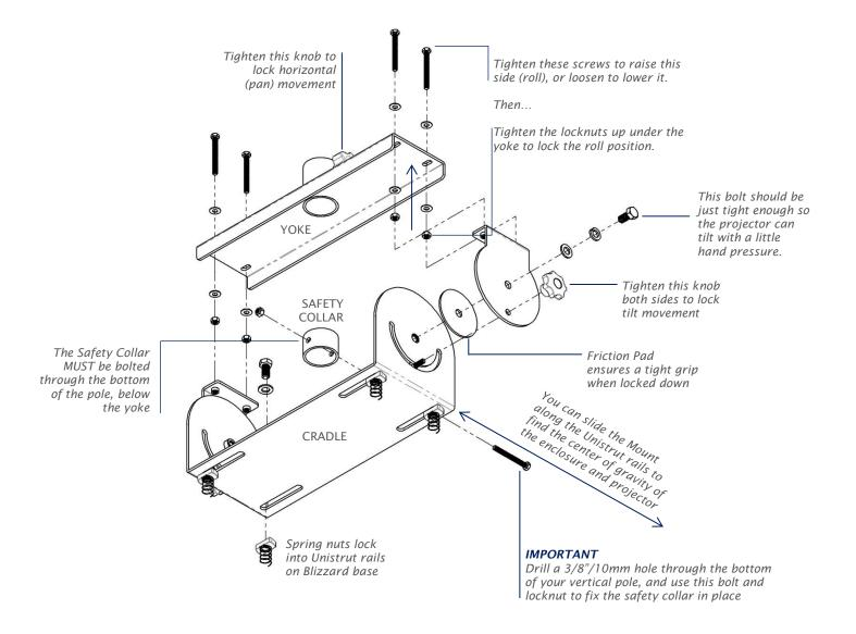
All Blizzard enclosures may be mounted using the adjustable Blizzard XYZ mount. The XYZ Mount is designed to mount on the bottom of a piece of 1½" schedule 40 pipe (48-50mm Outside Dimension).
