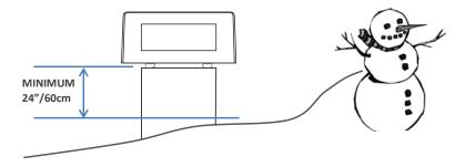
① Allow at least 24"/60cm clearance behind enclosure for access and ventilation (outdoor, Indoor).
