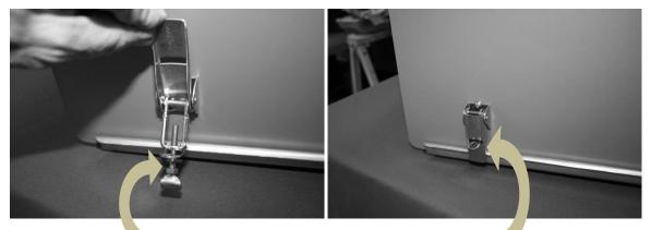
The latch tension is adjusted by turning the screw – clockwise to tension, anti-clockwise to loosen. Insert a padlock in one or more security rings for additional security.
