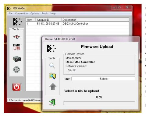
DEC3.3 firmware is fieldupgradeable, using RDM. A field upgrade requires a JESE RDM TRI MK1 interface to be connected to the DMX network on which the DEC3.3 is located, and the use of JESE GetSet software. The kit is available from Tempest under part # 2000.190.
