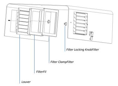
Remove any buildup of dust on the outside of the filter with a vacuum cleaner.
