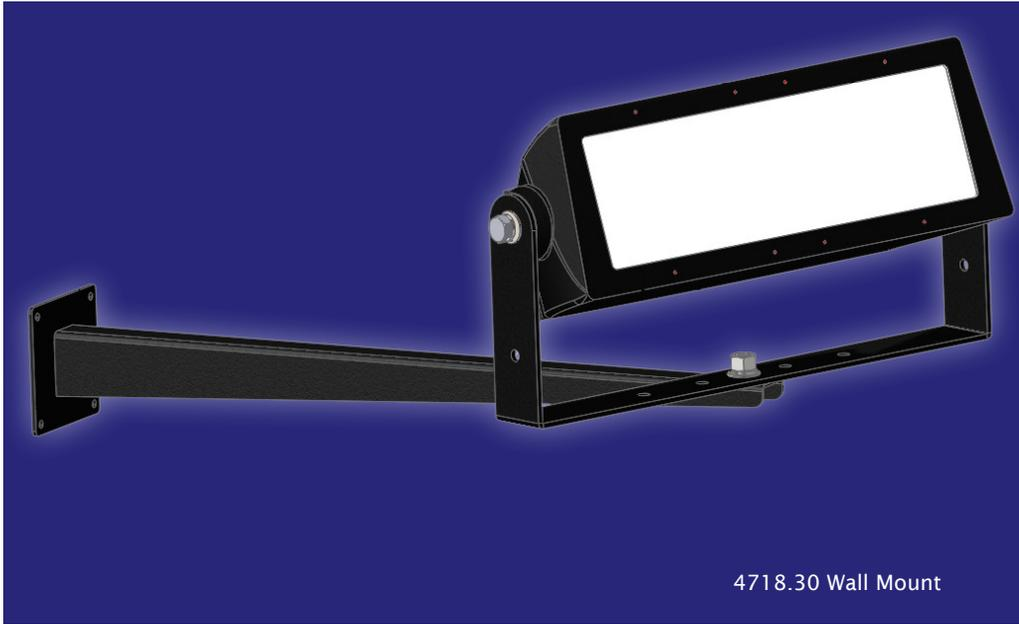
*These Wallmounts are made of rugged heavy gauge steel, plated for corrosion resistance and then treated with epoxy powder coat in a black texture to match the Compact Reach Luminaire.*
