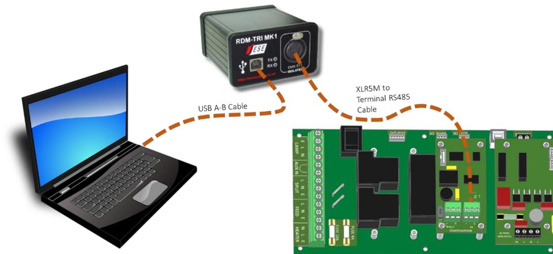
4. Power up the target SCB, ideally with mains power, or alternatively, with a USB power adaptor connected to the USB Port on the SCB.
