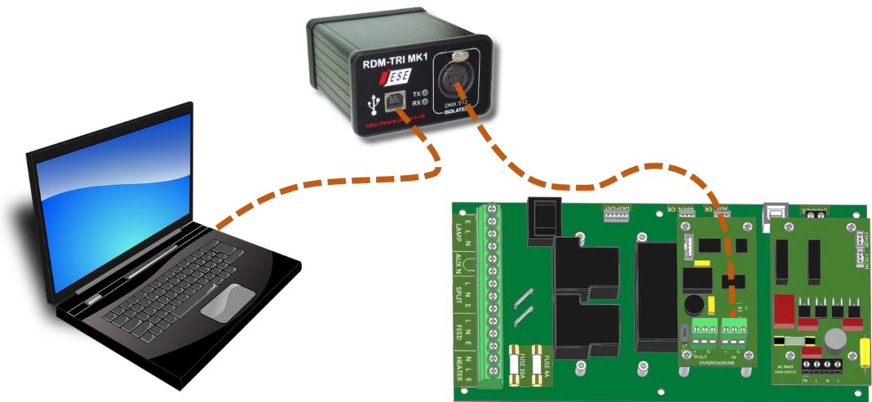
From time to time Tempest may introduce new DEC4 firmware for feature enhancements and bug fixes. Please note that the main System Control Board (SCB) and the various optional daughter boards each have their own firmware, and it will be good practice to update all firmware in an enclosure for optimal performance and interoperability.
