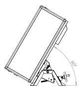
Note that as the required tilt angle increases, the enclosure is mounted progressively offcenter. This allows steep angles without requiring an excessively tall A-frame, and it also keeps the projector enclosure center of gravity close to the center of the Cyclovator. This is important from the point of view of minimizing image movement in crosswinds.
