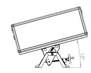
Illustration shows four angles, but any angle may be set and locked, between 0-60 degrees. Note the use of an Inlet Cowl to protect the inlet filter from rain when tilted above 40°
