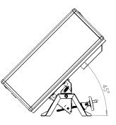
Cyclovator 2 is equally suited to projecting UP, with the front of the enclosure elevated, and DOWN, for example when the projectors are located on the top of a tall building.
